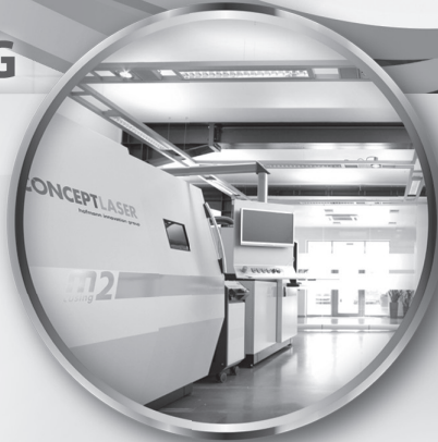
M2 CUSING SYSTEM Build Vol. 10" x 10" x 11" Single or Dual 200W or 400W Laser
